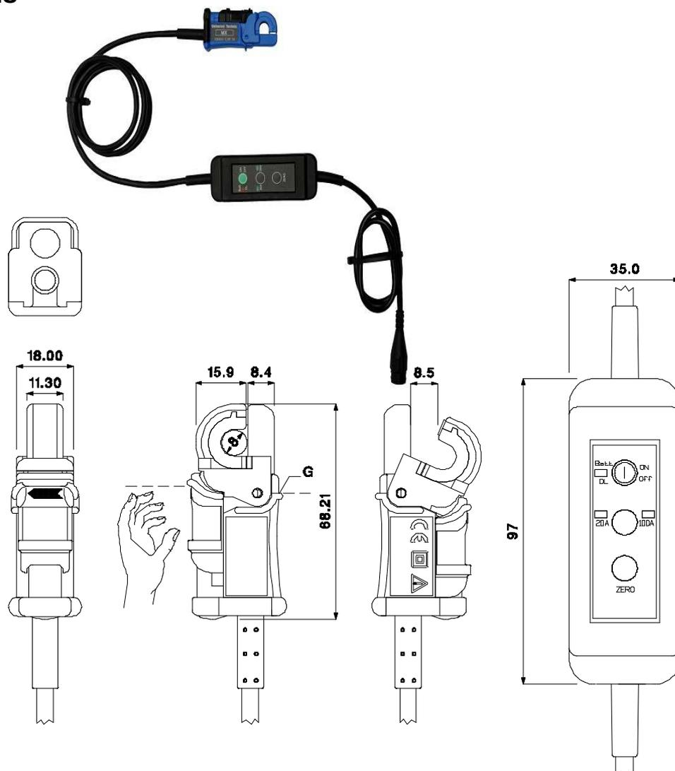
Length of cable : 1m from probe to control box and 50 cm from box to BNC output
