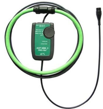
The new PRO~flex ACP 10000\_1 is an AC current Probe utilising the Rogowski principle. It can be used to measure currents up to 10000 Amps from very low frequencies to 10kHz. The flexible and lightweight measuring head allows quick and easy installation in hard to reach areas and with large conductors.
